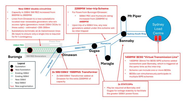
Option 5A is about using more capacity of the existing 500kV transmission lines using a SIPS scheme and then extra 330kV double circuit transmission lines within PEC to the generators:
