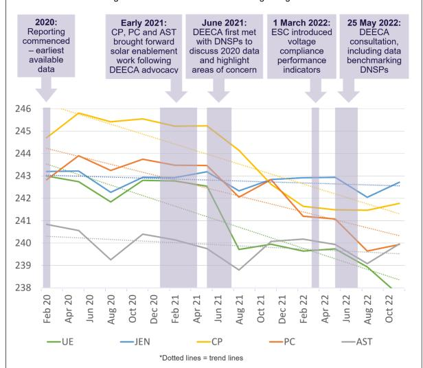
The data unequivocally showed that solar PV exports were not the primary driver of high voltage episodes. Instead, voltage spikes stemmed from network asset configurations and outdated regulation settings. Higher visibility allowed DNSPs to recalibrate transformer taps, manage regulator schedules, and improve on-load tap changer operations, reducing over-voltage incidents without curtailing solar exports.
