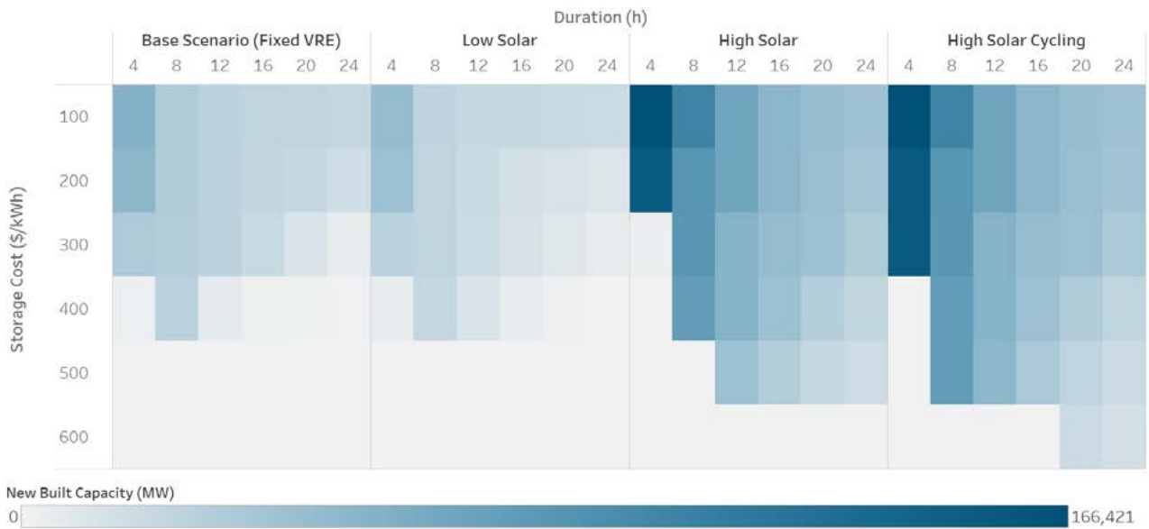
Figure 30: New ALDES build by solar build out scenario
